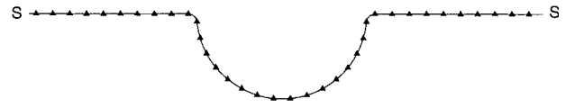
Fig. 2. In a typical simulation, the south boundary is represented by 400 evenly distributed points. Every third point is shown here.
